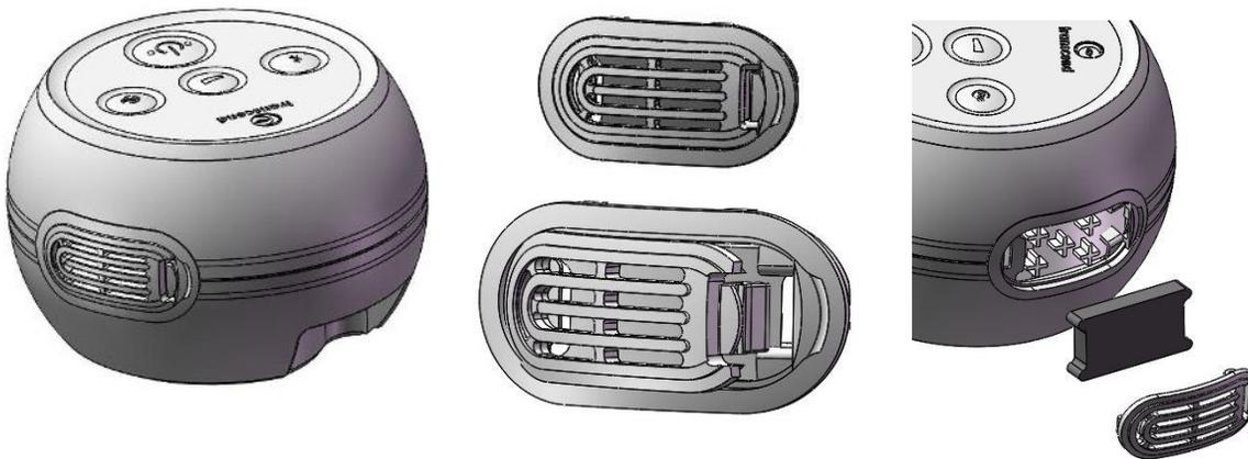
1. Depress the tab on the right side of the filter cover to remove it from the device
