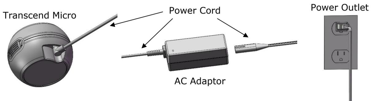
1. Connect the power cord from AC adapter into the power outlet at the bottom of the device.
