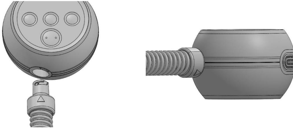
1. Connect the hose firmly to the air outlet on the device by inserting the hose coupler into the air outlet on the device.
