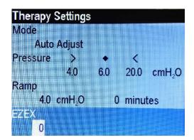
Push the Up or Down button to move the value from 0 to 3. A setting of 0 provides no exhalation relief, 3 provides the greatest exhalation relief. Press the Center button to save your selection.
