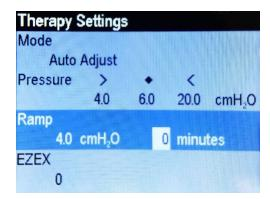
Use the Right button to highlight and the Center button to select Ramp Duration in minutes. Press the Up or Down buttons to change the duration from 0 to 45 minutes, moving through increments of five minutes. **Press the Center button to save your selection.**
