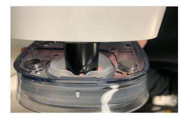
**NOTE:** In the case that the reservoir seal becomes dislodged from the reservoir, call your Transcend miniCPAP dealer for a replacement. If this occurs do not continue use of the humidifier as this may cause damage to your device.
