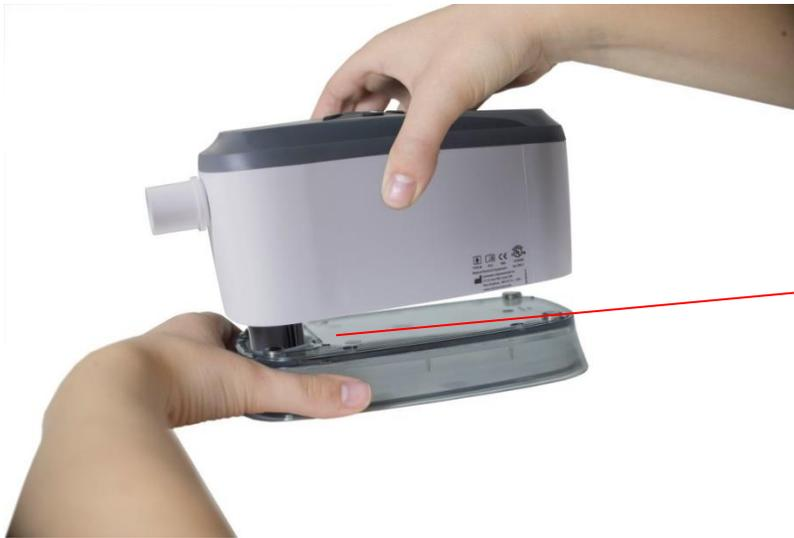
Line up the heater cartridge with the opening in the reservoir.
