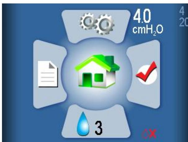
Indicated by a flashing red droplet and red 'X'. The humidifier will be disabled during therapy.
