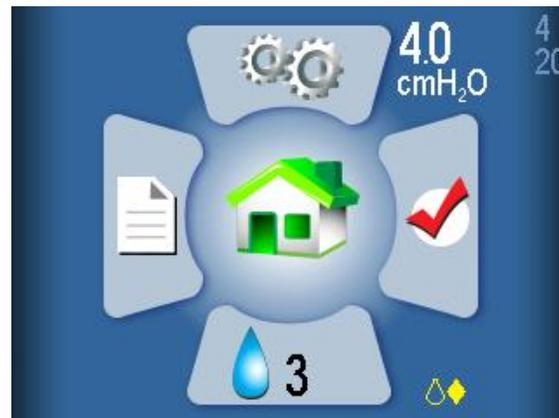
Only distilled water should be used with this humidifier. A flashing yellow droplet and yellow diamond indicate that water other than distilled water is detected in the reservoir. The humidifier can still be used, although doing so with any type of water other than distilled will shorten heater life and may void the warranty on the heater. This indicator may be caused by:
