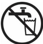
**Use distilled water only. The use of distilled water is required for proper function of the heated humidifier.** Failure to use distilled water will damage the humidifier and require repair or replacement. Alternatively, water may be filtered with the **Transcend Portable Water Filter** for use with your Transcend 365 miniCPAP humidifier.
