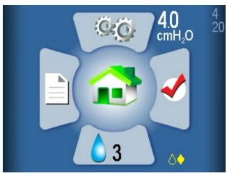
Only distilled water should be used with this humidifier. A flashing yellow droplet and yellow diamond indicate that water other than distilled water is detected in the reservoir. The humidifier can still be used, although doing so with any type of water other than distilled will shorten heater life and may void the warranty on the heater. This indicator may be caused by:
