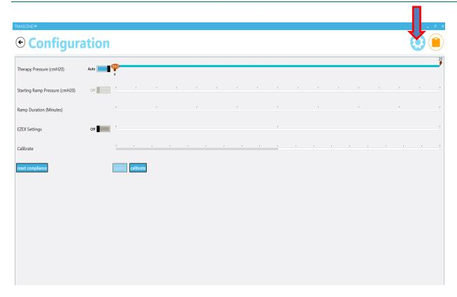
The Configuration area is used to adjust various settings on the device. Some features, such as the Therapy Pressure and Calibration are clinician settings and are only available with a password. You can, however, adjust the Starting Ramp Pressure, Ramp Duration and EZEX pressure relief settings if these options have been set by your clinician to be adjustable. To change them, simply slide on the red oval across the line to the right or left.
