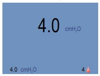
The red droplet indicates that the humidifier is not active. Normal CPAP therapy is not affected. This can be caused by any one of the following:
