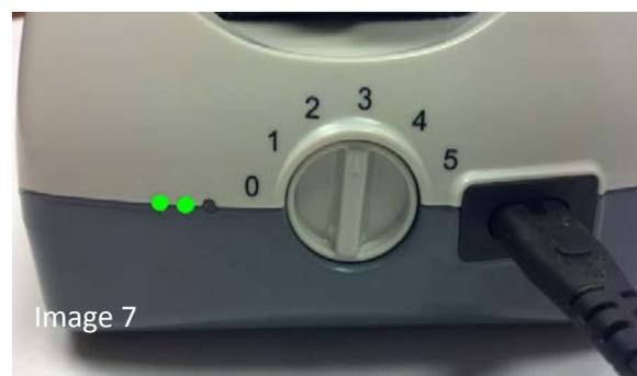
**Note:** The Humidifier will not begin warming the Water Reservoir until the PAP device power button has been pressed and the PAP device is in Therapy Mode. It may take up to 60 minutes to reach the set Humidifier temperature depending upon the selected heat setting.
