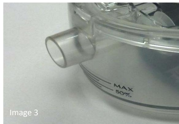
**Caution:** If the Water Reservoir is not fully inserted the heater will not activate and the rightmost LED will turn red.
