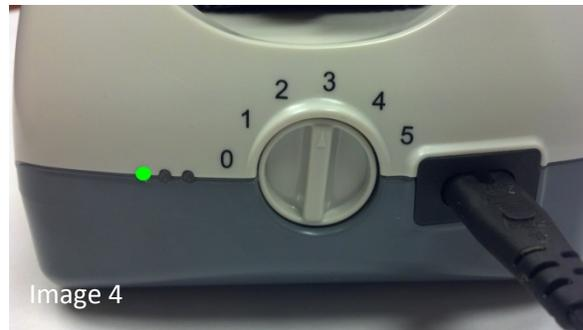
**Note:** When looking at the back of the device, the leftmost LED will turn solid green indicating that the Humidifier has power.
